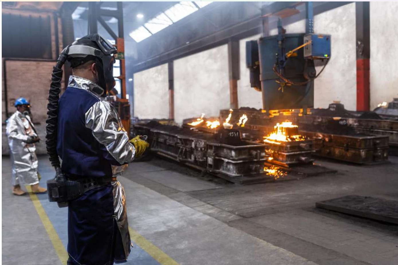
The project followed the full route from mould preparation to industrial casting and sand recovery.
