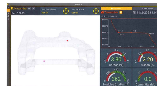
Fig.7 Real-time prediction of internal casting soundness. Simulation performed using the Kasandra® predictive simulation system
