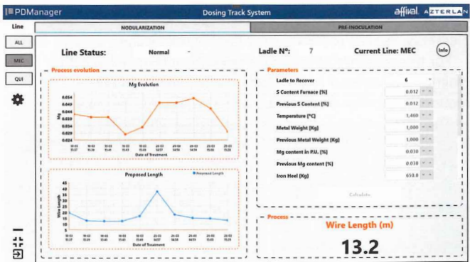
Fig.9 Calculation of the amount of Mg to be added based on data from previous treatments, carried out using AZTERLAN's Dosing Track intelligent system
