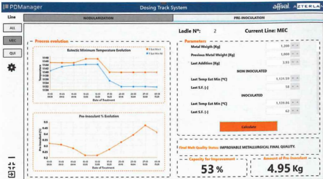
Fig.10 Calculation of pre-inoculation addition in the nodularisation treatment, performed using AZTERLAN's Dosing Track intelligent system
