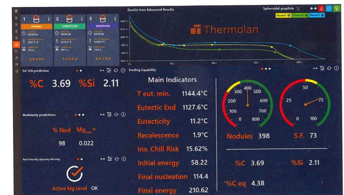
Fig.7 Example results for metallurgical quality control (GJS)
