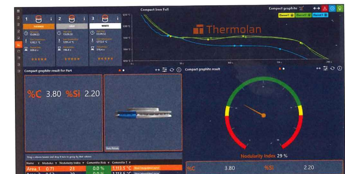
Fig.8 Results for metallurgical quality control of GJV, including extrapolation of results to specific areas of the component
