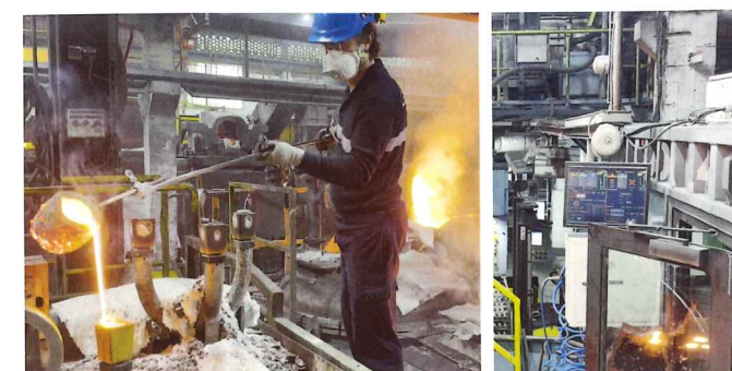
Fig.3 Typical application of a thermal analysis system on the melting platform, with on-site results visualisation
