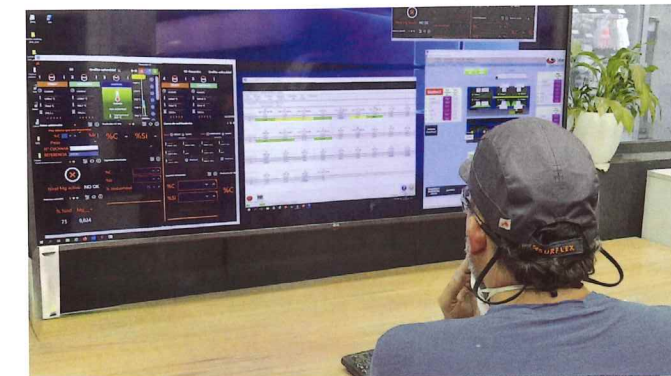
Fig.5 Thermal analysis results display (Thermolan®) integrated with other plant control parameters for process management and decision making
