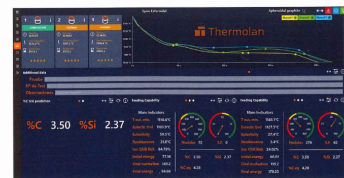
Fig.2 Main screen of a thermal analyser (in this case, Thermolan® system), showing the relevant parameters obtained from this analysis
