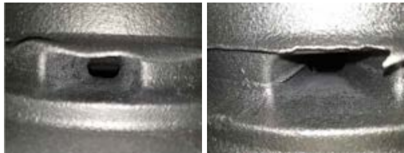
Fig. 5: Cast part from Fig. 4 after blasting: a) inorganic core without veining, b) PUR Cold Box core with veining.
