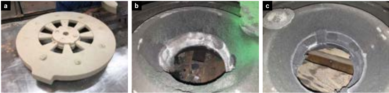
Fig. 4: a) Core for brake disk, approx. 15 kg, b) cast brake disk made of cast iron, inorganic core, sand adhesions, c) cast brake disk made of cast iron, PUR cold box core.
