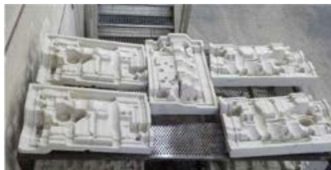
Fig. 7: Inorganically bonded core package cores for iron casting.
