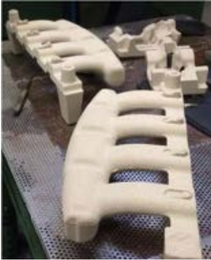
Fig. 8: Inorganically bonded intake manifold cores for non-ferrous casting.
