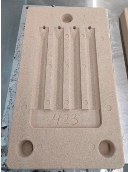
Lower part of the sand mold
