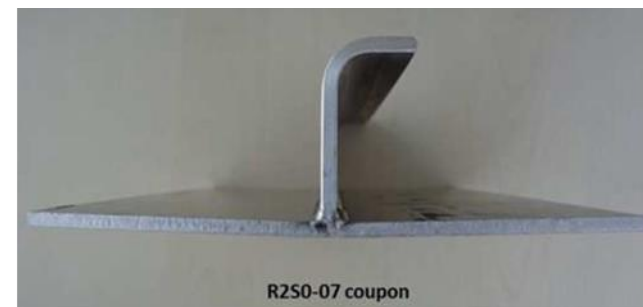
1 stringer type: L formed: R1, R2, R3, R4 & R5
