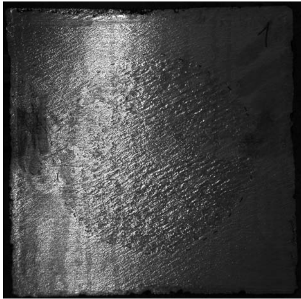
Fig. 1—Central section of a cubic block (30 cm in size) with the zone affected by CHG appearing with darker contrast.
