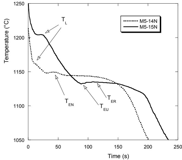
Fig. 2. Cooling curves recorded from the TA cups cast with non post-inoculated #14 and #15 melts. The characteristic temperatures considered in this work are indicated. As no recalescence showed up during the bulk eutectic reaction of M5-14N TA-cup, the  $T_{EN}$  and  $T_{EU}$  values were taken equal to the temperature at the inflexion point at the very beginning of the eutectic plateau.
