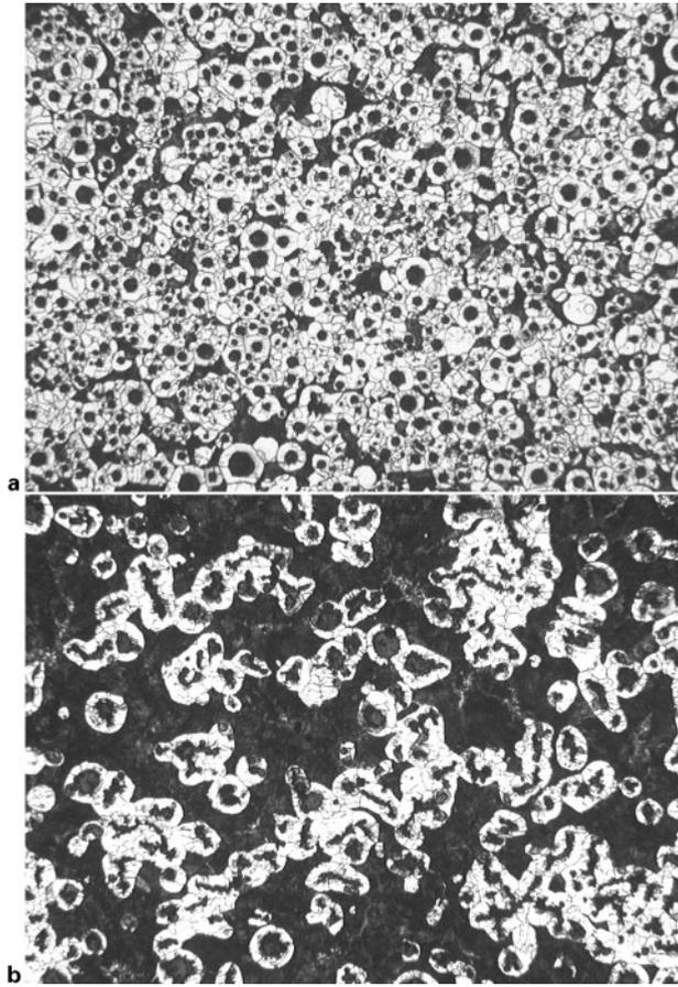
7 Microstructures of a inoculated and b non-inoculated samples in test 1-1,  $\times 100$
