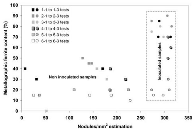
**6 Ferrite evolution in inoculated and non-inoculated samples analysed in present work**
