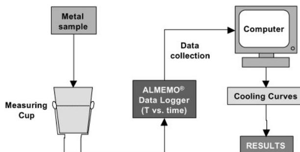
3 Scheme of thermal analysis system used in experimental measurements
