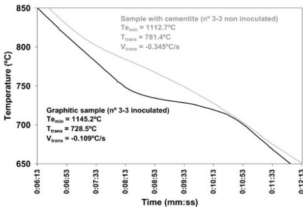
8 Comparison of eutectoid transition in white and graphitic cast irons
