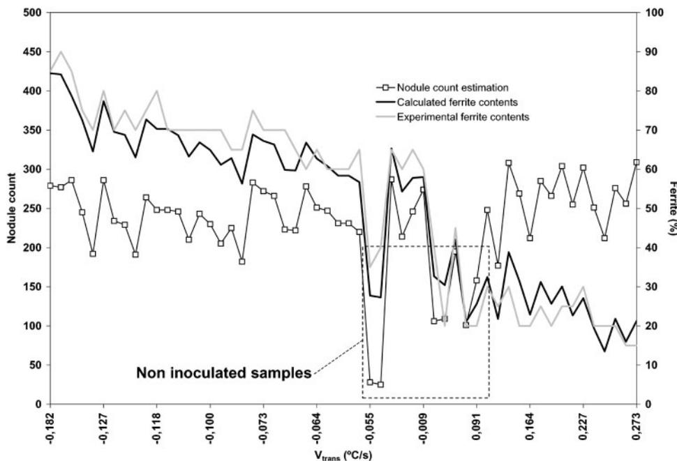
10 Comparison of experimental and calculated values of ferrite contents
