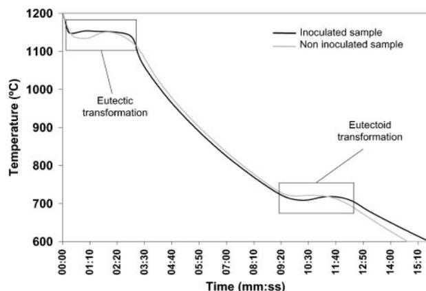
1 Cooling curves for inoculated and non-inoculated nodular iron samples
