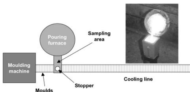
2 Scheme of moulding line and sampling method
